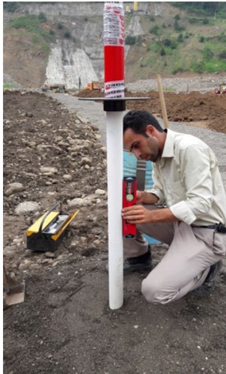
Inclino-settlement column with magnet plate - Polrood Dam
