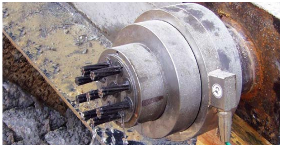
Sisgeo's electric load cell with load distribution plate
