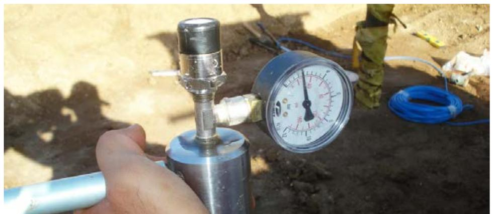
Saturation of HAE filter with saturation device
