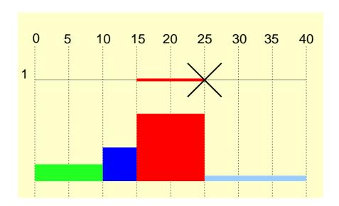
In the graph above power use is estimated assuming that at time 25 the Modbus master has sent a switch-off command.
