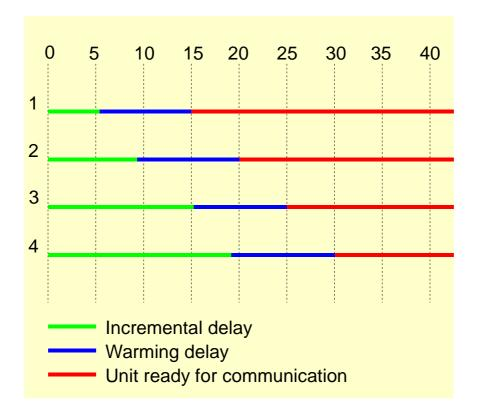
During the delay time, instrument and AD are powered, so that this accounts as settling time for the measure. It is expected that the Modbus master will send a switch off command after reading the instrument so that power drain will switch to a minimum.
