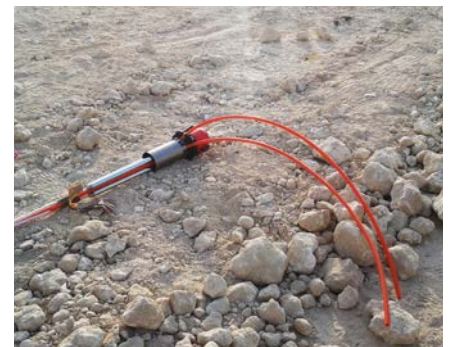
Sisgeo extensometer head ready for installation
