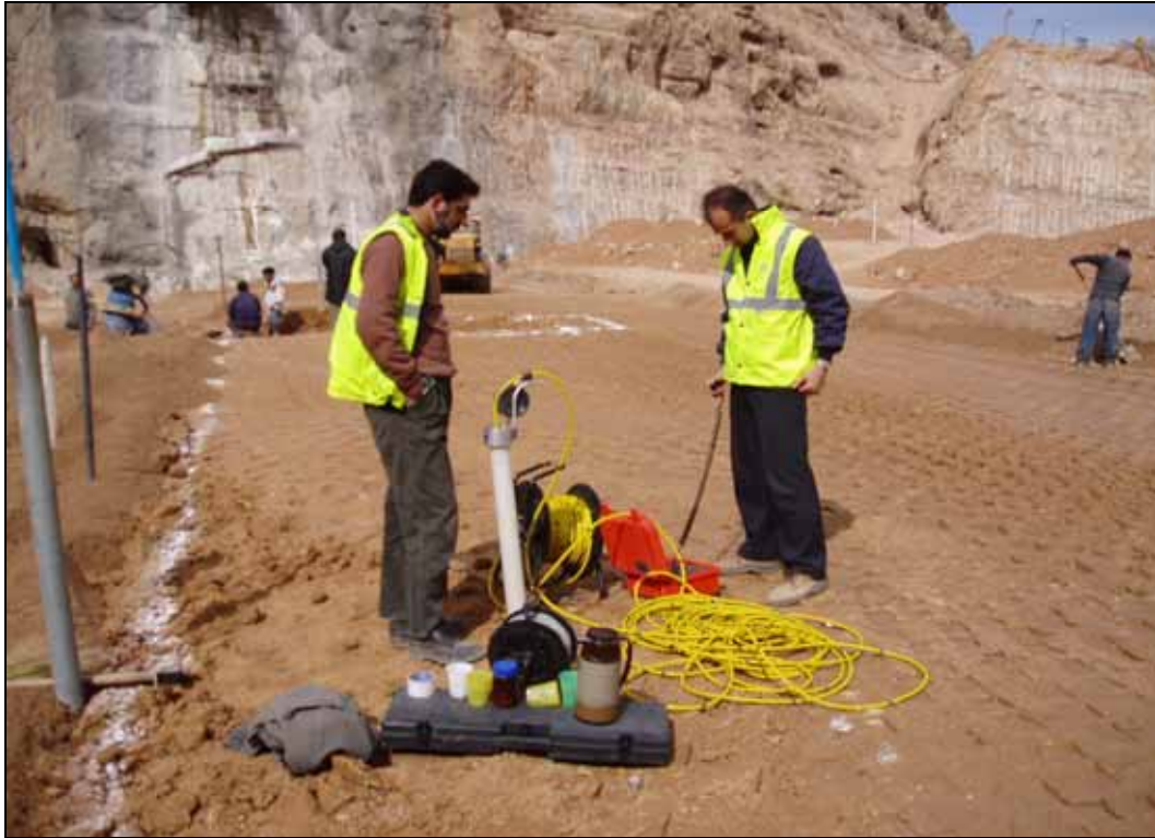
Vertical inclinometer measurements
