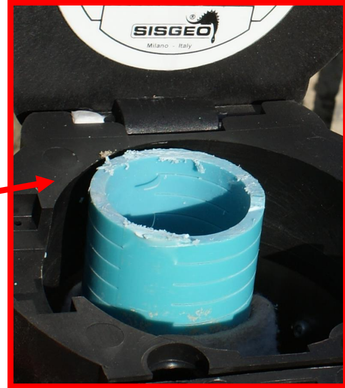
Stand pipe piezometer head: detail of slotted tube with geotextile filter
