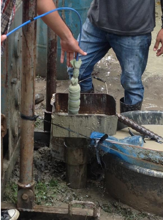
Insert the transducer in the borehole
