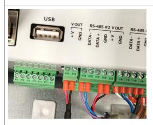
The power cable provided must be connected to the OMNIALog terminal block, in the V OUT section, as follows:
