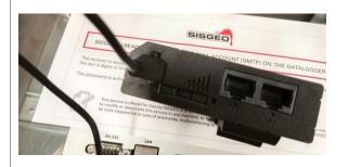
Then the other side of the power cable must be connected to the router as in the picture
