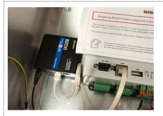
Insert the router onto the cabinet flange so that the router part with the antenna connectors is facing upwards. Press down firmly to lock the router in place until you hear a CLICK.
