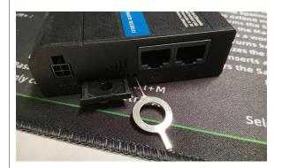
To insert the SIM card (not supplied by Sisgeo), open the SIM card slot as indicated in the picture
