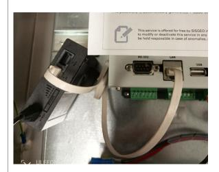
Now connect one end of the LAN cable supplied inside the cabinet to the "LAN" port on the OMNIAlog, and the other end to the "LAN" port on the router (do NOT connect the cable on "WAN" port)
