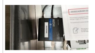
Last step: connect BOTH antennas to the two connectors labelled as "MOBILE" on the router as shown in the image. The antenna cables must pass through the lower cable gland on the cabinet. The antennas must be positioned so as to have a signal strong enough for data transmission.
