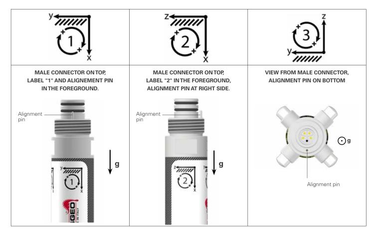
If the gauge is installed e.g. in a **horizontal tube** such that the y-axis is vertical and parallel to g, the data returned by the gauge will be on channel 1 (XY plane <u>rotation</u>) and channel 3 (ZY plane <u>rotation</u>), while channel 2 will return no data (channel automatically disabled as described before for the vertical application).
