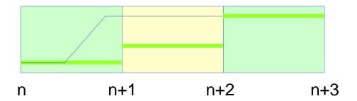
In the above graph, the thin line represents the input value and the green line the moving average. It can be seen that the moving average settles up to two periods after the input value has changed: any change occurred during the period starting at time 'n' is only completely accounted for at time 'n+2'.
