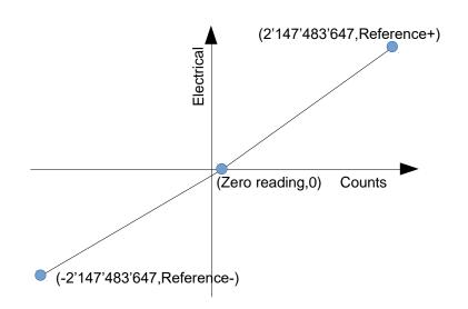
The conversion is linear in both ranges (Zero reading, 2'147'483'647) and (- 2'147'483'647, Zero reading). The two lines can have slightly different slopes.
