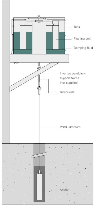
The inverted pendulum provides a fixed datum from which structural movements can be measured. It is composed by:
