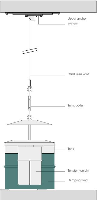
The direct hanging pendulum is a gravity-referenced instrument consisting of:
