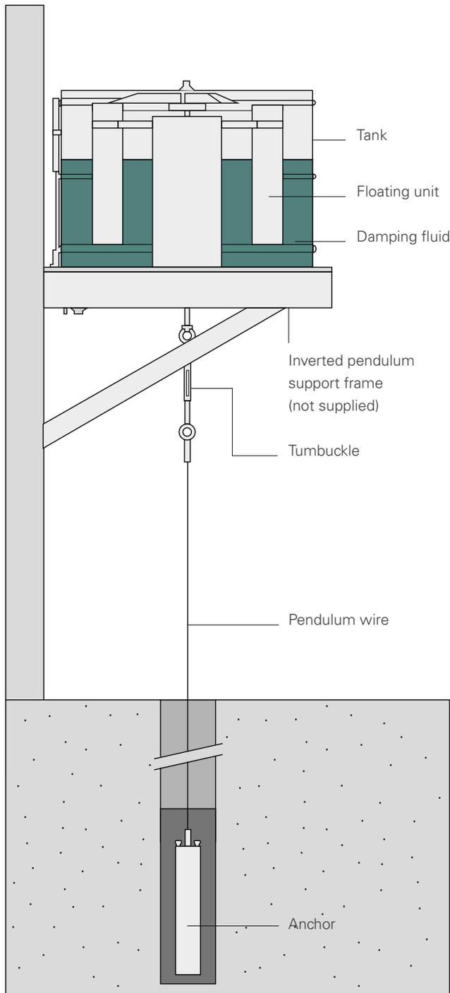
The inverted pendulum provides a fixed datum from which structural movements can be measured. It is composed by:
