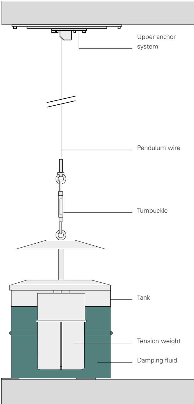
The direct hanging pendulum is a gravity-referenced instrument consisting of:
