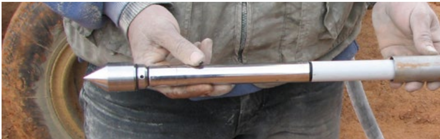
Drive-in piezometer with push-in rod
