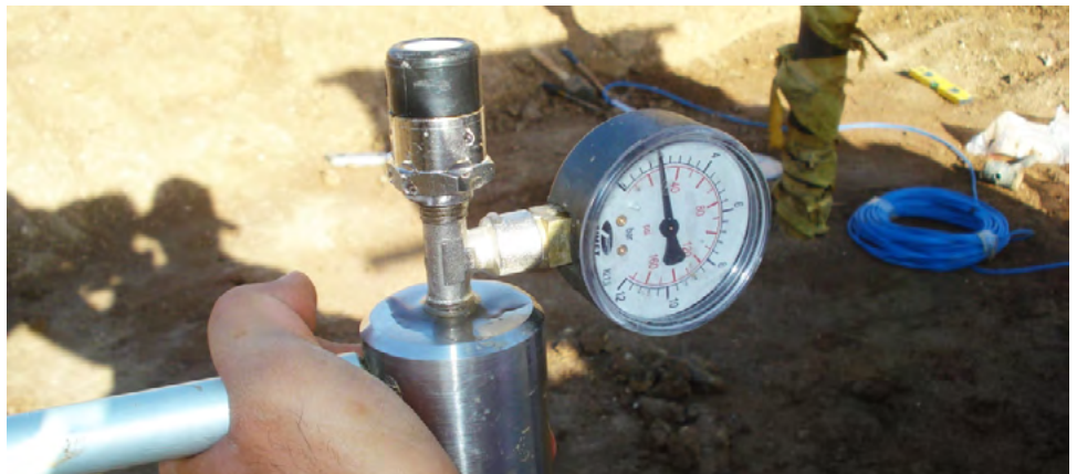
Saturation of HAE filter with saturation device
