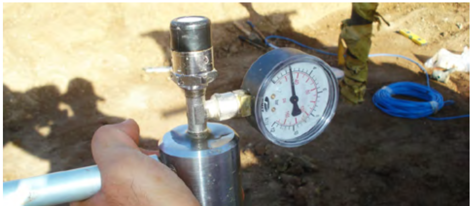
Saturation of HAE filter with saturation device
