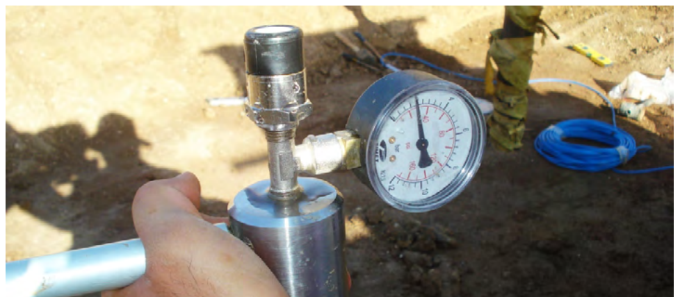
Saturation of HAE filter with saturation device
