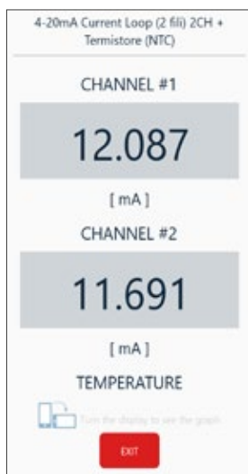
Instrument reading page with both biaxial 4-20mA current loop channels reading. The temperature measure is displayed scrolling down.
