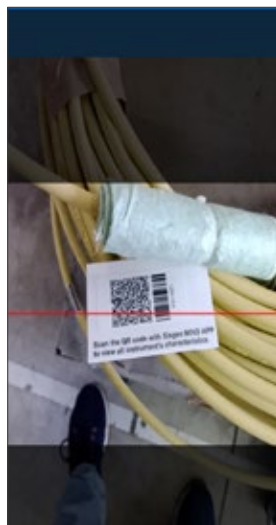
QR code scanner for automatic configuration of analog sensors.
