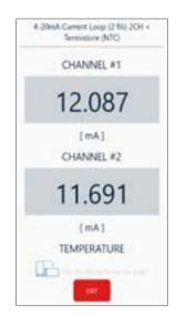
Instrument reading page with both biaxial 4-20mA current loop channels reading. The temperature measure is displayed scrolling down.
