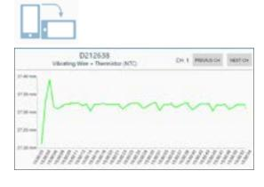
Graph of connected sensor's readings. It is generated just turning the mobile device in horizontal position.
